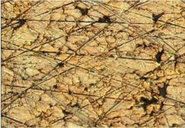
圖 7: P1-Fig.7 The as-cut surface of a porous sintered bronze part taken directly from a precision wafering saw.
