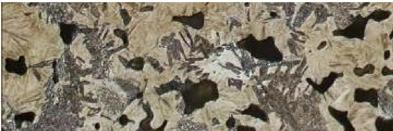
P2-Fig.1 Hybrid alloy using a pre-alloyed low-alloy steel base containing (wt%) 0.4 Mn, 1.25 Mo, & 1.4 Ni with 1 wt% elemental Cu + 0.7 wt% graphite additions (FLC-4805). Sintered at 1120° C without accelerated cooling (2 vol% Nital + 4 wt% Picral)
