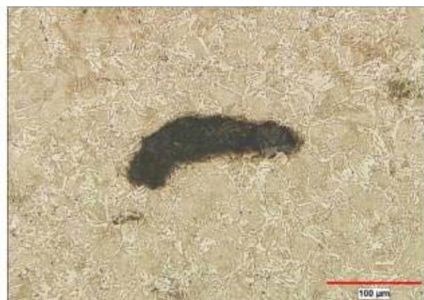
**P2-Fig.9** An unalloyed Fe particle shown as a darkened feature in a pore-free, powder forged low alloy steel (2 vol/o nital + 4 wt/o picral then Beraha' s 3-10)
