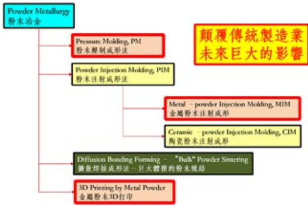
圖 2：第五代的金屬成形製程區分 Classify of the 5th generation of metal forming process
